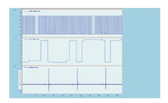
The high-speed Snapshot Mode captures the complete signal envelope, buffering and transferring this to the data logger via the CAN interface. The built-in display is another helpful feature which allows the module to be used as a hand-held assistant, even when data logging isn't required and a computer isn't used.
